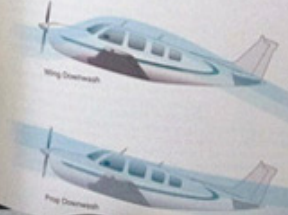
Figure 3-36. The downwash from the propeller and the wings passing over the horizontal stabilizer influences the longitudinal stability of the airplane.
